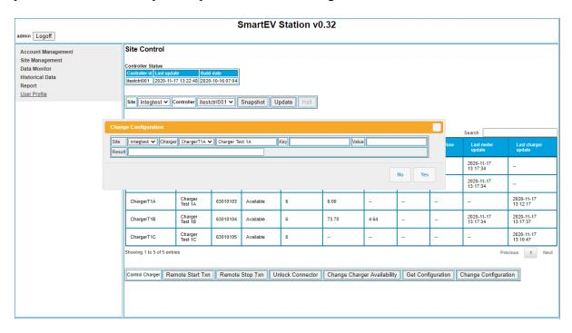
For real time monitoring and control, the system facilitates data and control command over secure streaming protocol over 4G mobile or LAN network. Electric current and charging status can be viewed per station controller.
