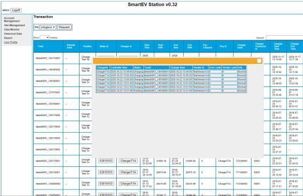
Although only one meter consumption can be displayed, data export provides all metering consumption during transaction. These kinds of information provide background study on how effective the power management module and also as the criteria of upgrading electricity supply.
